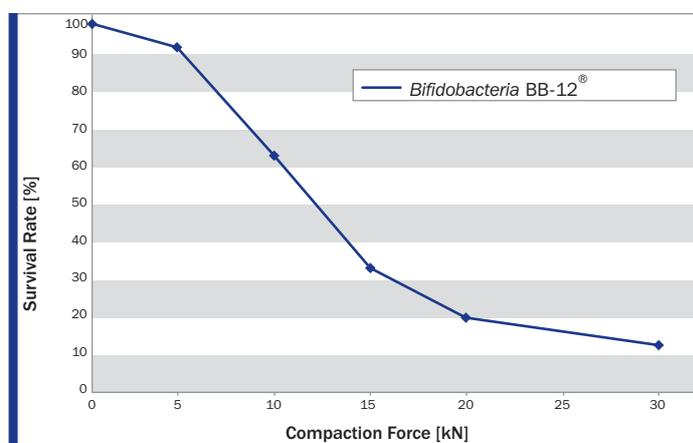
Fig. 1 Correlation between Compression Force and Viability of Bacteria Cells in Directly Compressed Probiotic Tablets Containing 20 % of the *Bifidobacteria* Strain BB-12<sup>®</sup>.
