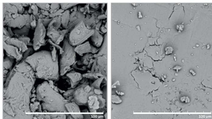
Pic. 1 Tablet Surface of Probiotic Tablets with a Crushing Strength of 80 N Containing PROSOLV® EASYtab Nutra (left) and Spray-dried Lactose (right), Respectively.
